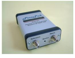
The new PicoPak Module is a small and inexpensive USB instrument for making precise phase and frequency measurements on clocks and oscillators.
